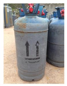
However, once the cylinder is placed on the back of a Fork Truck, it is essential that the bottle is rotated until the arrows on the side are facing vertically upwards – as shown below:
